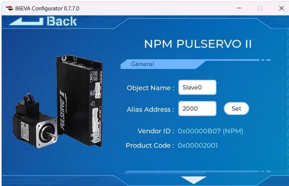
The page will show the Object Name, Alias Address, Vendor ID, Product Code, Virtual Arduino Mapping, and Virtual Servo Configuration parameters.
